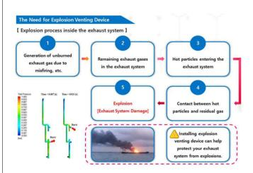
The characteristics of Explosion Venting Device are as; The safest explosion protection device that instantly releases the maximum amount of explosive expansion gas and pressure, and blocks flame and releases only pressure and smoke. It is leak-free and non-fragment design, and blocks the temperature inside the exhaust pipe. In addition, the initial product price is low and there are no separate maintenance costs and real-time status monitoring possible by applying an integrated sensor disc.
