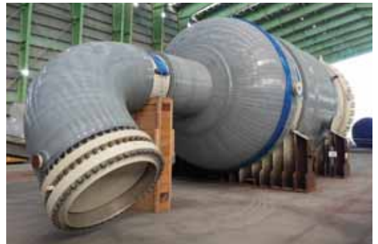
Vessel Insulation for FLNG Top Side
