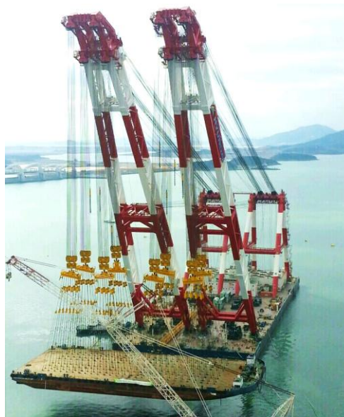
10,000 ton Floating Crane Wire Reeving and Commissioning
